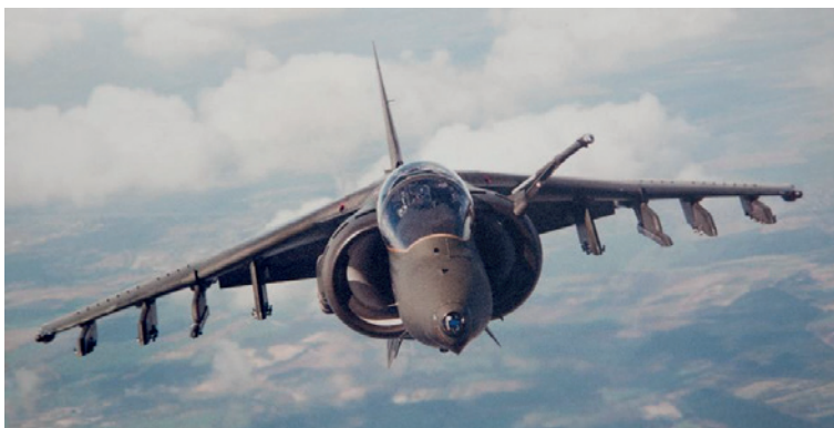
A GR5 second-generation Harrier with its powerful Rolls-Royce Pegasus engine – here with its air-to-air refuelling probe extended.'
